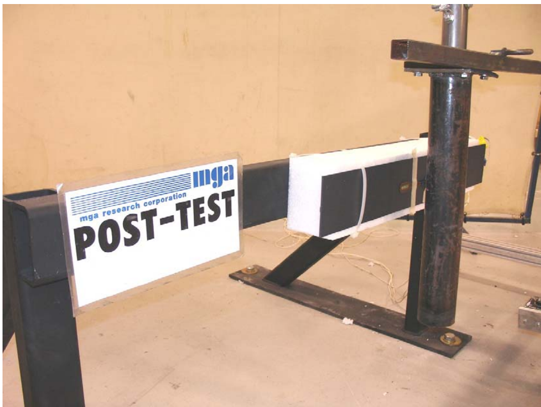
Photo No. 2 – Pendulum Impact System Set-Up
