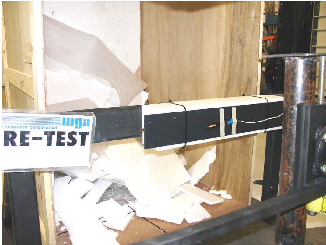
Photo No. 1 – Linear Impact System Set-Up
