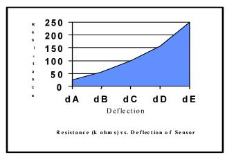
The rate of change as displayed in the graph is dependent on two factors. The first is the bend radius, the smaller the radius the greater the change. Secondly is the angular deflection. For a given radius the more the sensor is bent around it the greater the change.
