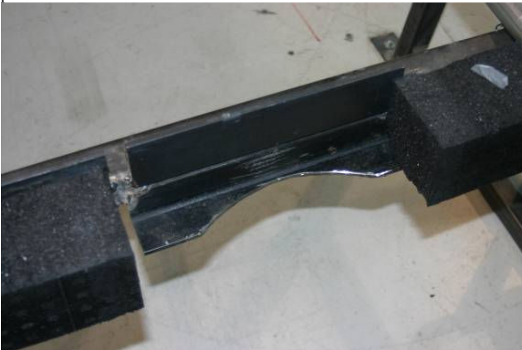
Figure 4: The angle iron block support was relieved to prevent damage to the leg and pole during impacts.
