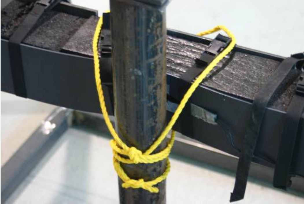
Figure 3: Unloaded bumper block. The indentation is from the repeated impacts, the sensor still performed well.
